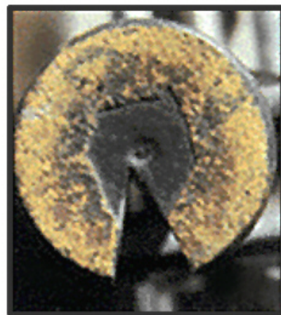
Figure 6: Tetraethyl lead corrosion on an exhaust valve head face caused by fuel oxidized by the combustion process forming lead oxide deposits on the valve head.
