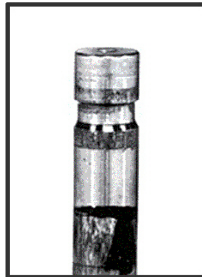
Figure 3: Chafe marks at the side of the groove indicating that the valve has been bouncing instead of following the cam
