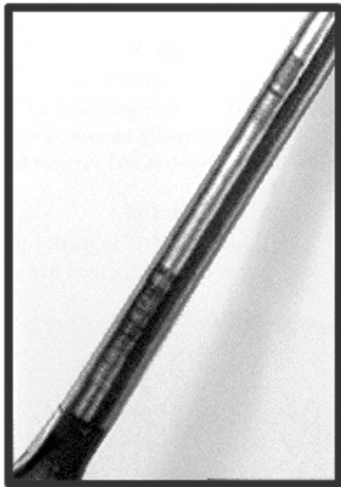
Figure 5: Contact patterns on a valve stem indicating its movement within the valve guide.
