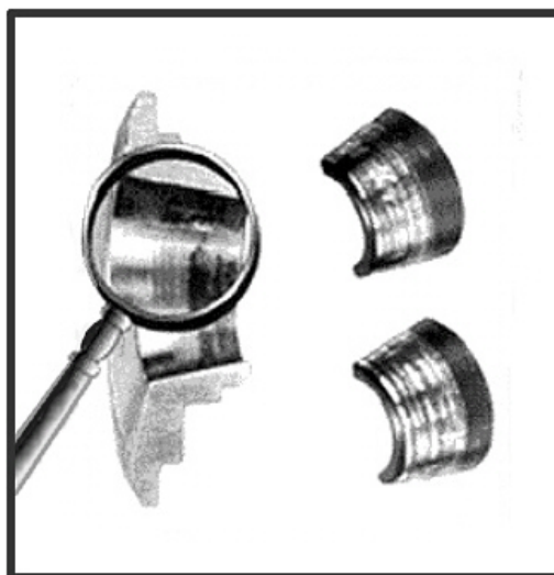
Figure 4: Circumferential chafing pattern on both the spring retainer and the valve keys indicating movement relative to each other during operation,
