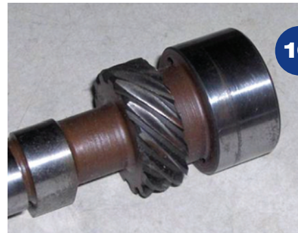
Fig.10: Cam drive gear wear
