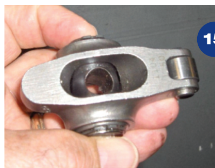
Fig.15: Fulcrum mounted roller rocker
